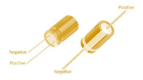
Fig. 1.1.18: Polarity in electronic components
