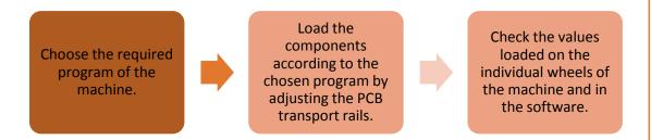
Fig. 2.4.19: Steps for loading the components into the feeder
