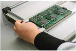
Fig. 2.4.13: Positioning of the circuit board
