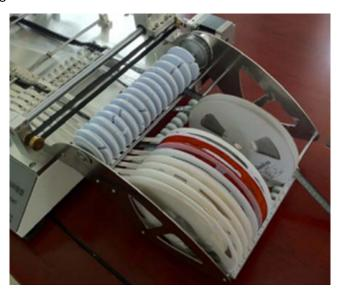
Fig. 2.4.6: Reel rack of a pick and place machine
