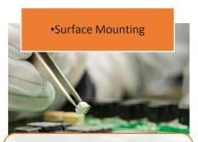
•This mounting method is used in the case of components which are very small in size. For example, this method can be used to mount components which are the size of a pencil point onto a PCB.
