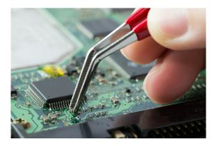
Fig. 1.2.11: Mounting components onto a PCB
