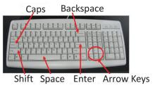
Fig 5.2.2 Basic parts of a Keyboard
