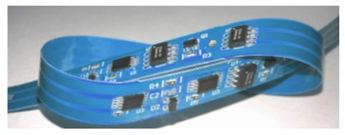
Fig. 1.2.8: Flexible PCB
