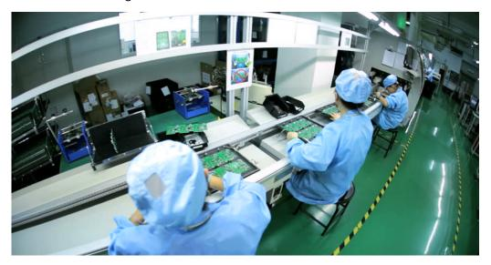
Fig. 1.3.11: PCB manufacturing
