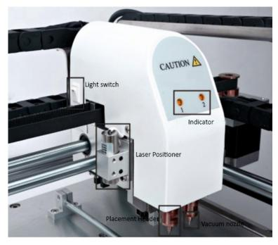
Fig. 2.4.3: Working heads of a pick and place machine
